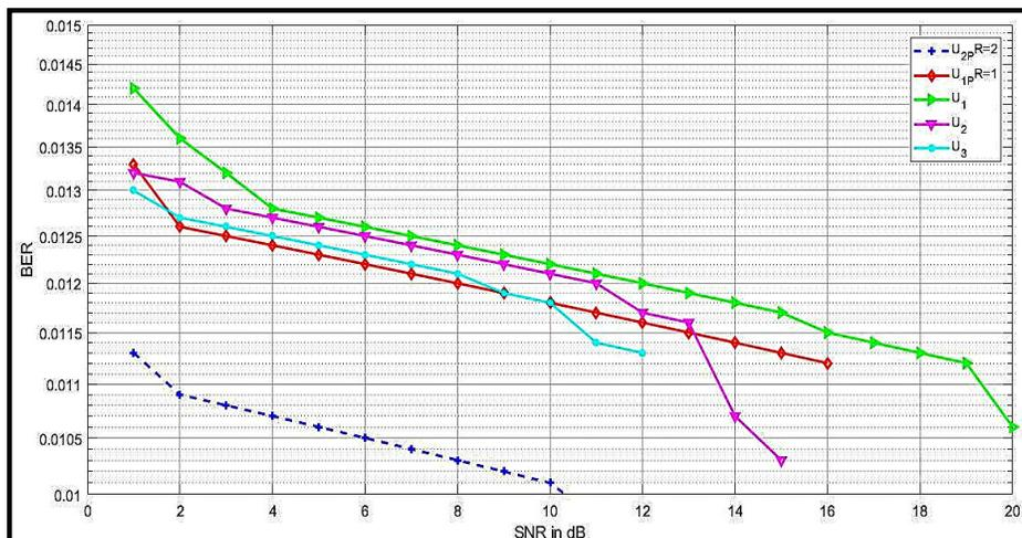
**Fig. 6.** BER performance of Modified  $\mu$  law companding technique on SCM-OFDM system with different companding levels  $U_1, U_2$  and  $U_3$ . Table IV: Comparison of PAPR Reduction techniques for SCM-OFDM system.
