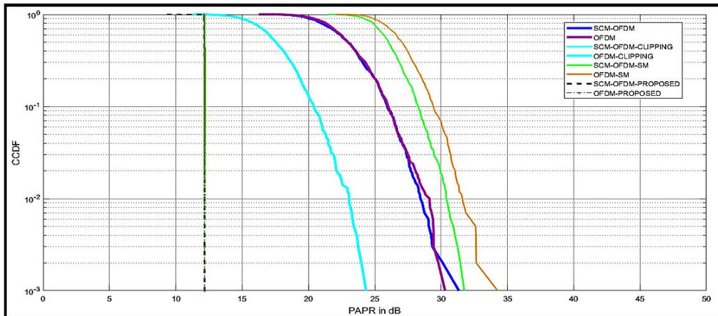
Fig. 9. Comparative study of PAPR on SCM-OFDM systems for 256 QAM modulation with different reduction techniques.
