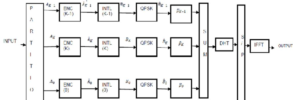
Fig. 1. The Proposed SCM-OFDM system for PAPR reduction.
