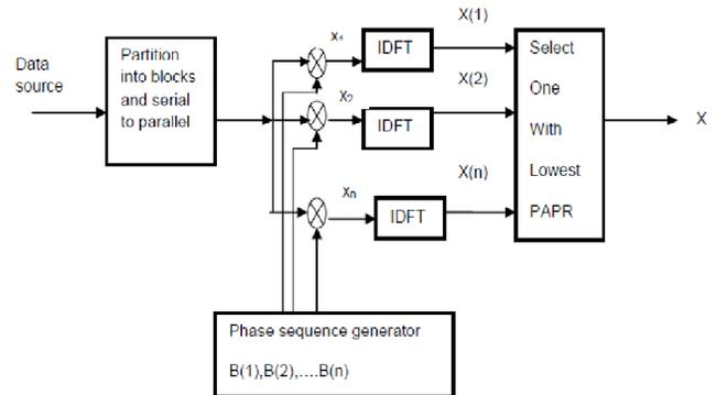
Fig. 2. Block diagram of Selective Mapping.
