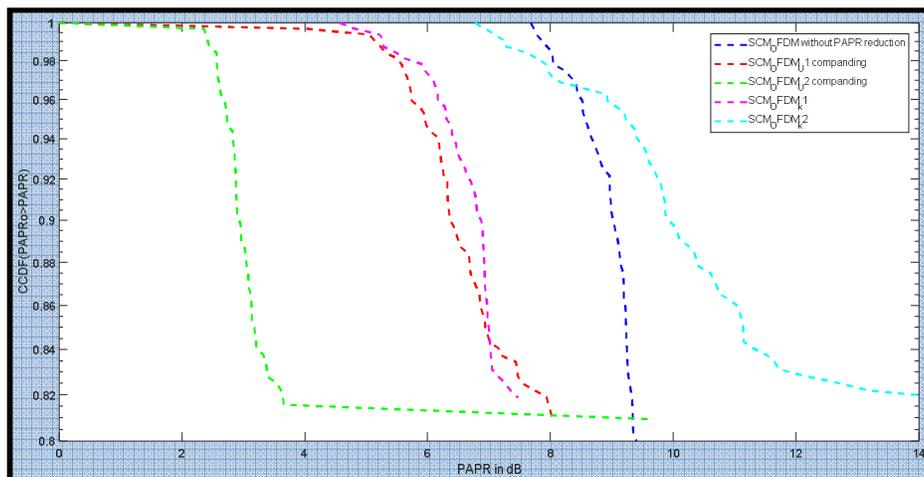
**Fig. 5.** CCDF Vs PAPR for different  $\mu$  companding profiles ( $u_1, u_2$ ) and modified  $\mu$  companding techniques.
