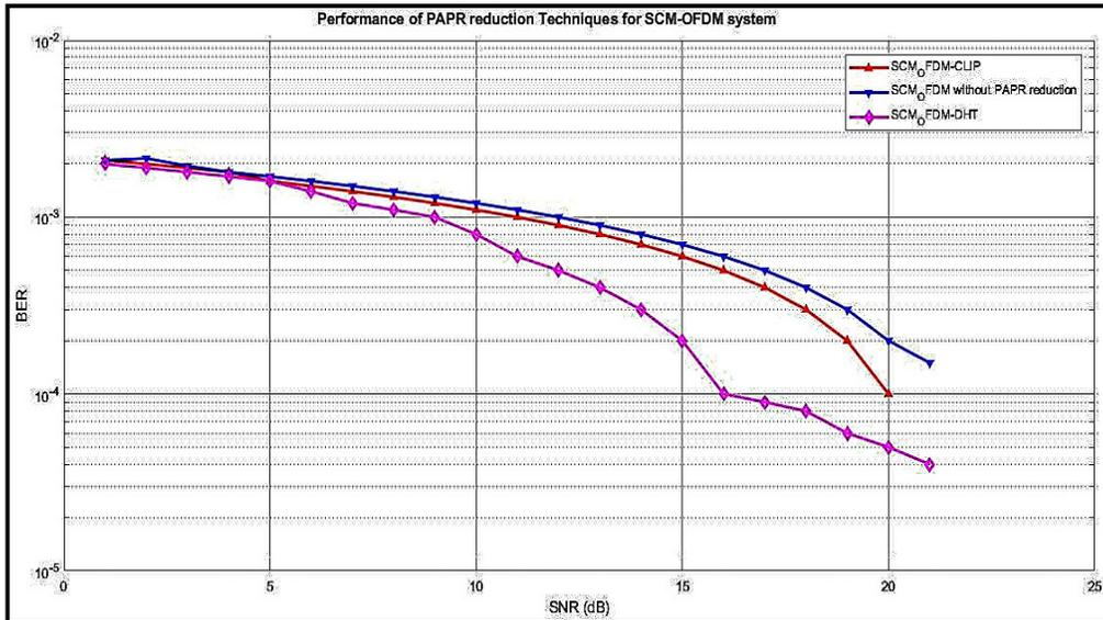
Fig. 4. BER performance of Clipping and DHT PAPR reduction techniques in SCM-OFDM system.
