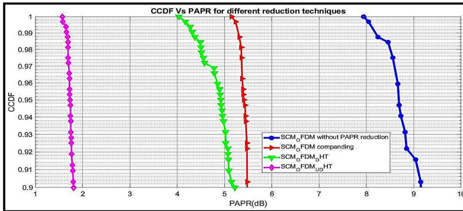
Fig. 7. CCDF Vs PAPR for different PAPR reduction techniques on SCM-OFDM system.
